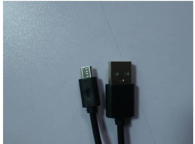
44. Charging cable terminals
