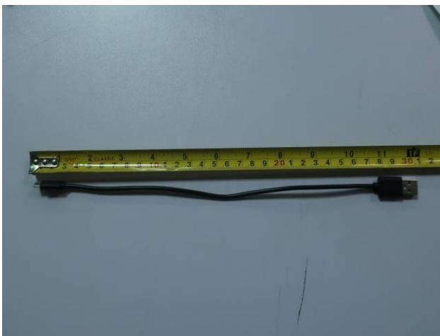
45. Charging cable length check
