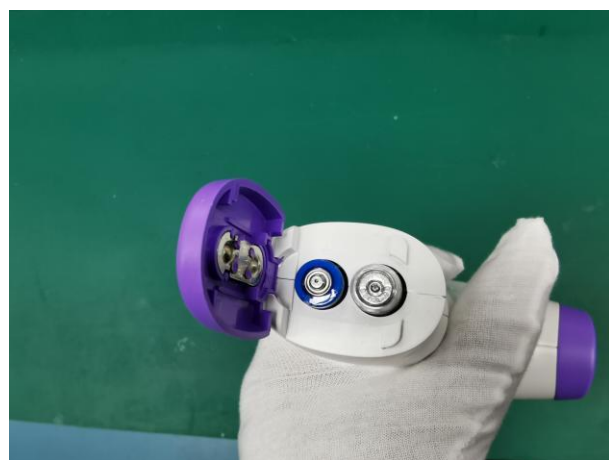
41. Battery fitting test
