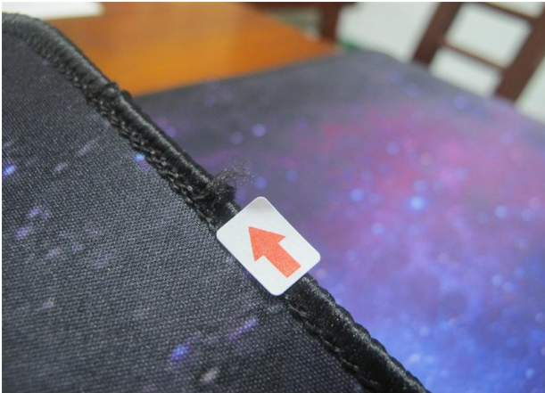
3 Defect: Poor trimming on the end of band (Minor)
