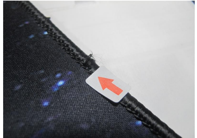
4 Defect: Poor trimming on the end of band (Minor)
