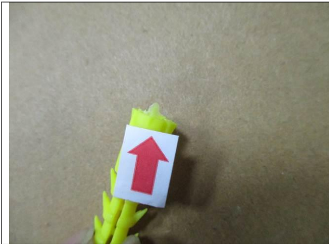
00 defect-flash on plug (1)
