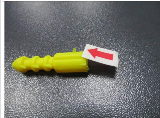
00 defect-flash on plug (3)
